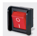
C1553AA with M616 guard Cut-out 22.0/22.1 x 29.4/29.5 Guard accepts "A" body only
