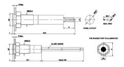
6mm Vandal Resistant Indicator LED Colour LED Voltage Material Series Diameter Termination DX 06 - 6mm W - Wire Leads 200mm R - Red 006 - 6V N - Nickel Plated Brass L - Solder Lug G - Green 012 - 12V B - Black Plated Brass Y - Yellow 024 - 24V S - Stainless Steel B - Blue 110 - 110V W - White 220 - 220V
