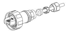
Slide gland, gland cage and gland nut up to body moulding then tighten to torque of 1.5-2.0lb/ins. 13-18Nm.
