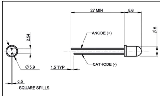
**Figure 2: new led specification**
